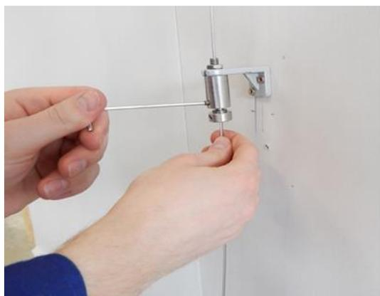
8. Loosen upper screw (locking movable part of the tightener).
