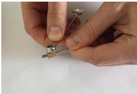
1. Before cable guides installation, put sleeves on the cable guides.
