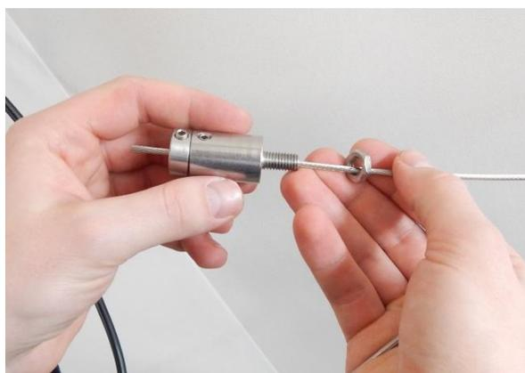
5. Put cable through façade tightener.
